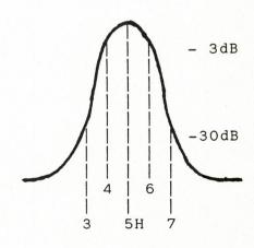
This menu point is for shifting the harmonic which the rub and buzz filter is tracking. The harmonic for the filter shifts when the menu point is selected. The filter can be set up for tracking from the 1st harmonic (fundamental) and up to the 12th harmonic.
