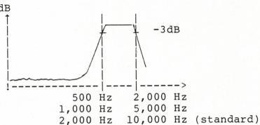
The gain in filters and maximum frequencies displayed for different filter settings with a band pass filter installed:
