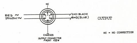
Pin 2 and 4 are shorted internally Pin 1 and 5 are shorted internally
