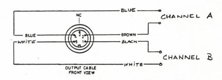
WARNING! CVA2 outputs are floating. Do not short output to ground.
