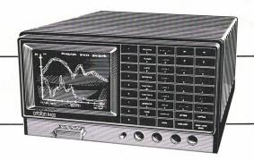
Telephone transducers operate both as receivers and microphones. The measurement of the frequency response/sensitivity, rub & buzz/distortion and impedance characterize the acoustical performance of the transducer. Furthermore, the loudness rating is calculated from the frequency response measurement using a small external computer and additional software. The test cycle is typically 3-6 seconds. Two (2) test stations can be controlled by one (1) P 400 Measuring Computer.
