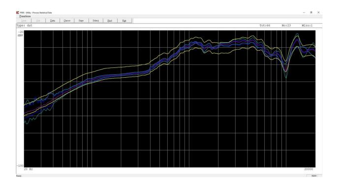
The same data is now processed. Displayed are the upper and lower limits, the average of collected and selected data and in this case +/-3 Standard diversions (sigma). With benefit the upper and lower limits could be modified. I would use +/-3 sigma and add a limit example +/-1 db to this.
