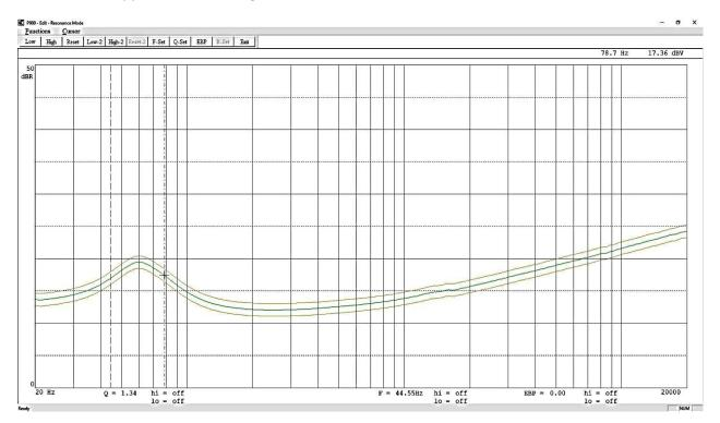
Test envelope for Frequency response is used +/- 3 db. In this case the sensitivity has to be within this envelope.
