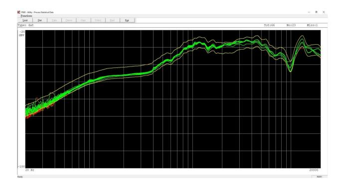
In this example above show only the frequency curve data processed in manual mode. Number of collected measurement is in this case 23 out of 66 measurements. This show that the current limits could be fitted better to the measured data.
