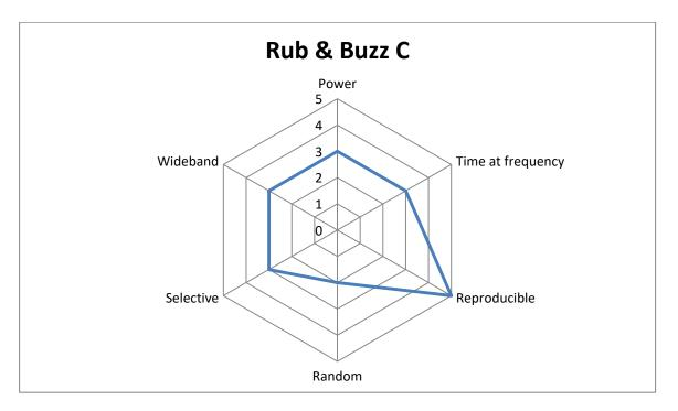
D) Buzzing signal as selective resonance generated due to some missing gluing. Medium predictable, medium or slow test speed, some power depended. The selective resonance generated due to missing glue need to be energized. So this is time and power depended. Faster test more power etc.
