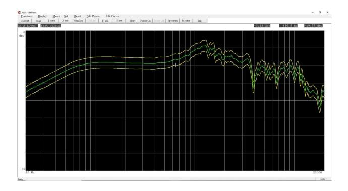
In the following example only frequency curve limits are used. The limits are moved +/-3.1db. Normally higher tolerances are given at the lower and higher frequency due to wider deviations.
